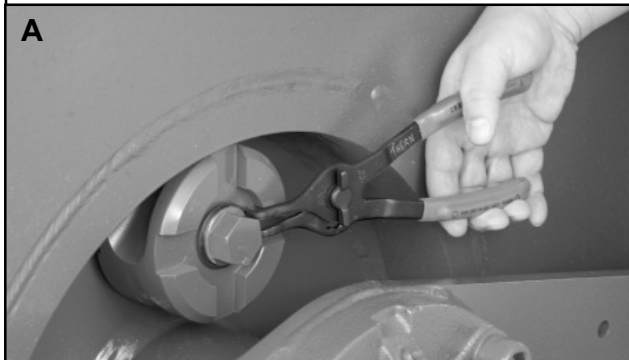
Figure 8 – Reversing the Cable Anchor
